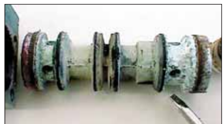
Contaminants corrode and damage air-operated equipment
